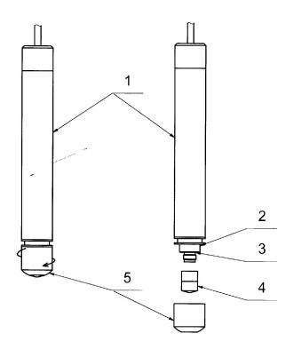
Fig. 1 Sensor CSOT 63-88 – exchange of membrane head
