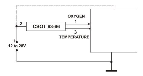
Fig. 2 Sensor connection to external device
